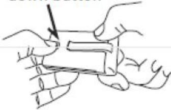
While holding down the button, slide the cover in the direction shown
